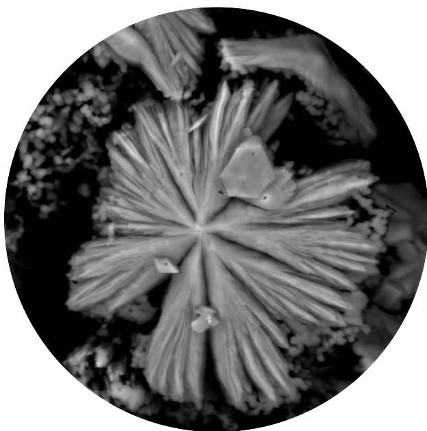
Untreated limescale: needle-shaped, intergrown dendrites that adhere to surfaces.
